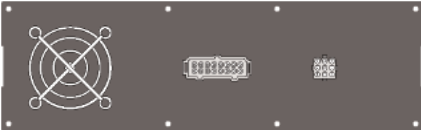
2 x AMP (9P - 25A) - DMX connector (DDK) at the rear - Supply HARTING. For use in MEMORACK 180
